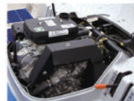
Water-cooled 3 stroke diesel engine (PZ60AD/PZ60DT/PZ80-25/PZ80)
