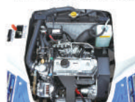
Water-cooled 3 stroke diesel engine (PZ60AD/PZ60DT/PZ80-25/PZ80)
