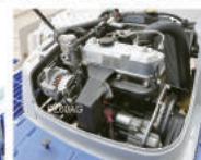
Water-cooled 3 stroke diesel engine (PZ60AD/PZ60DT/PZ80-25/PZ80)
