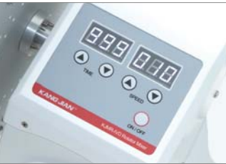
LED with backlight can display the current speed, time and operation mode, convenient for readingand setting.
